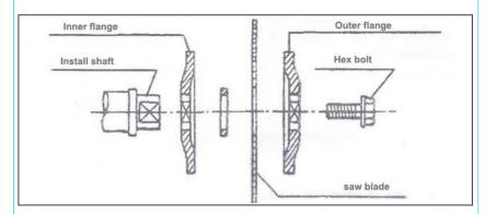
Install the outer flange and the hex bolt. Then, press down the shaft locking arm,and tighten the hex bolt firmly by turning it counterclockwise using the socket wrench,then adjust the hex bolt in clockwise so as to fix the central cover.
